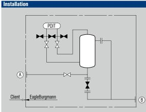
P&ID for LSB6000-A4 Leakage collection system A From mechanical seal B To liquid collection system
